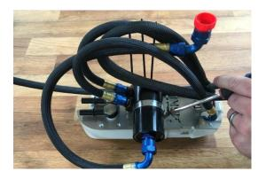
Remove filter housing from Jubilee Clip and layout as shown
