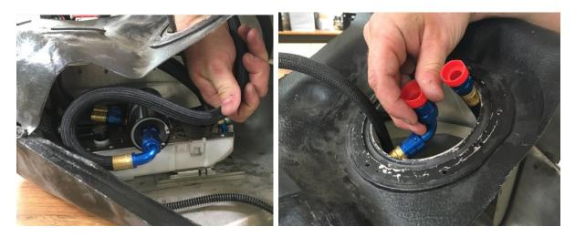
Connect pump connectors to the top plate assembly , these can be connected either way round
