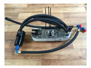
Using long nose Pliers spread return line and insert original fuel return line regulator and scavenge pipe work, and then fit to basket module.
