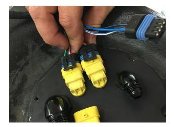
Unwind main harness assembly - the long section of wiring with a fuse box at the end requires a battery main feed it is designed to be run along the door sill under the carpet up the bulk head and thorough the firewall to the battery compartment, the fuse box can be disconnected to allow the wiring to pass through the bulkhead. There are 2 additional wires for additional ASNU upgrades that are not used these are left un-terminated (black with blue trace & green).
