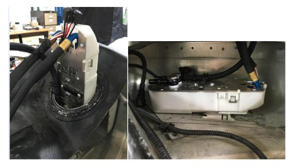
Lock tank module into the base of the tank,
