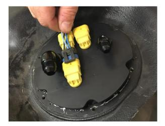
Connect twin short connectors as shown these are not orientation sensitive (shown with level sensor plug off for clarity). These are the primary and secondary pump connectors
