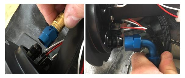
Lay top plate into place ensuring the correct orientation and tighten the fittings
