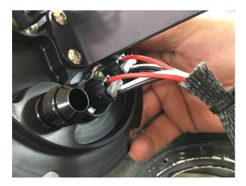
Fit tank level sensor to sender arm, trim original plug off. Using supplied 4 pin connector connect red to red & black to black on the sensor ves the 4 pin connector adjacent to the sender arm . if a tank temp sensor is fitted connect one black wire and the other to the white wire. And then fit the sensor bulb into the basket.
