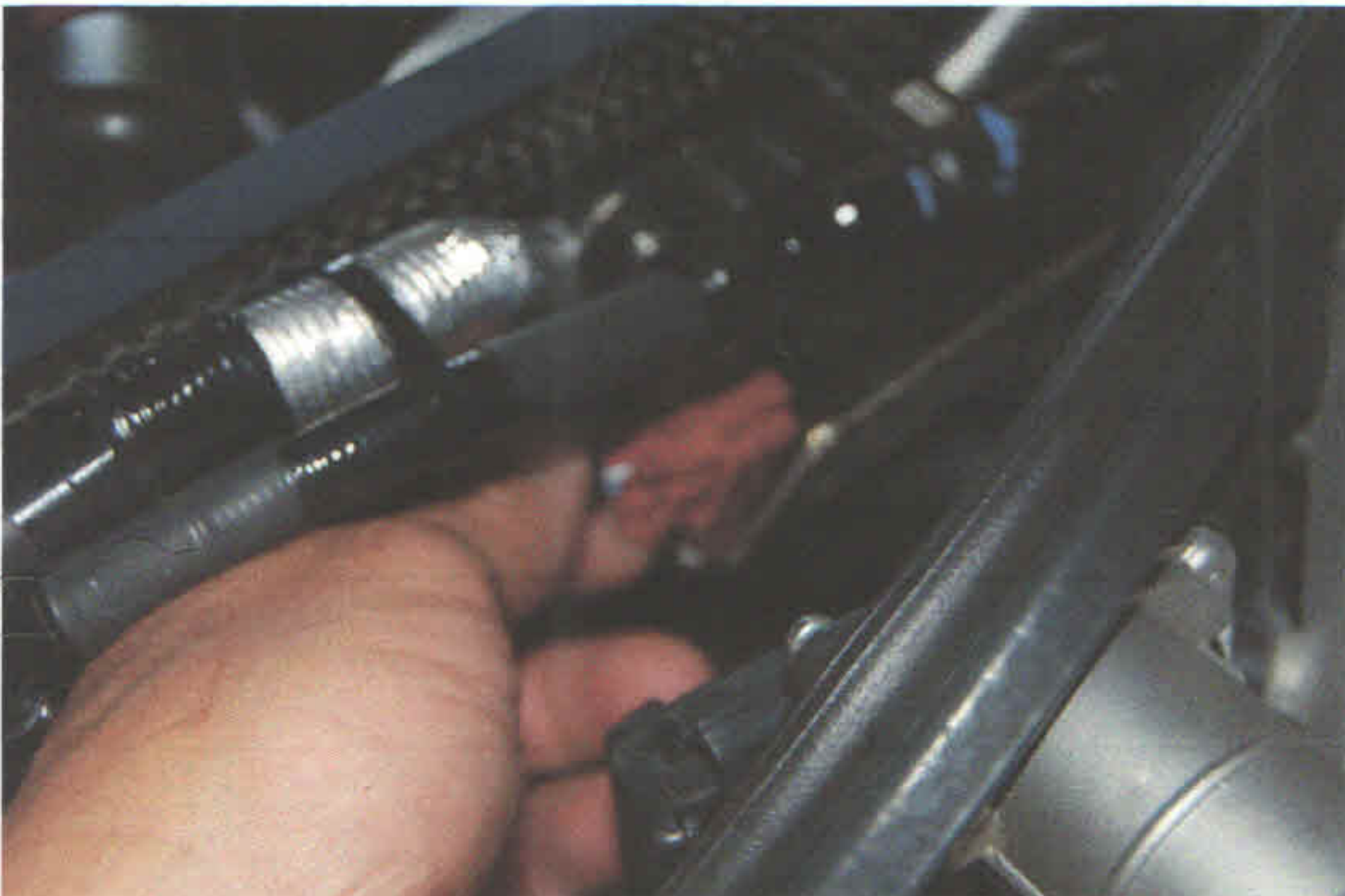
Connect brown plug on Flex Harness into the Flex Fuel sensor.
