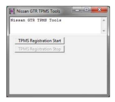
Using the widely available Nissan TPMS it's now possible to reset the TPMS light. Start the registration sequence then visit the indicated wheel and press the button on the handheld TPMS tool for registration. Please contact if you would like to purchase one
